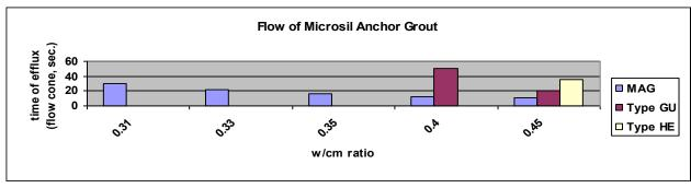
Type GUL Cement below w/cm of 0.45 is not fluid enough to pass through a flow cone. Only M.A.G. is fluid and pumpable below a w/cm of 0.4.
