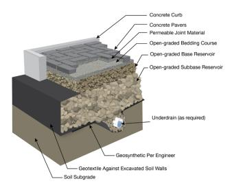
Figure 1. Typical permeable interlocking concrete pavement cross section.
