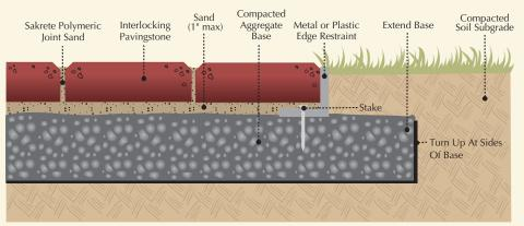
Note: Thickness of compacted aggregate base will vary with subgrade conditions and climate. Colder climates may require thicker bases.
