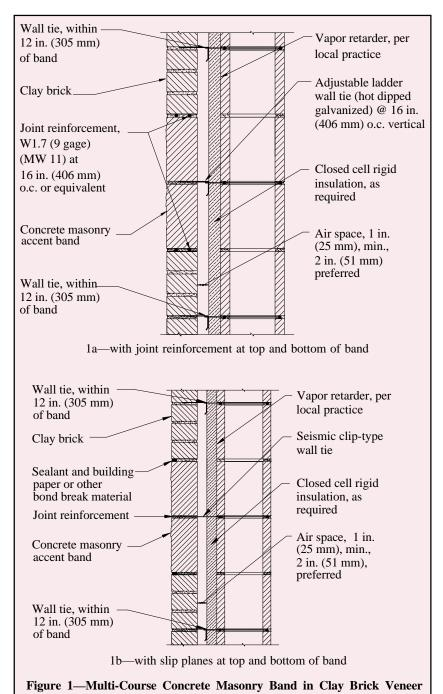
reinforcement continuous through that joint. The continuous joint reinforcement in this location helps keep the clay brick above and below the band from cracking as the concrete masonry shrinks.
