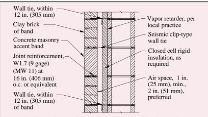
Figure 2—Single-Course Concrete Masonry Band in Clay Brick Veneer
