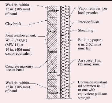
Figure 3—Concrete Masonry Band in Clay Brick Veneer Over Wood Stud Backup
