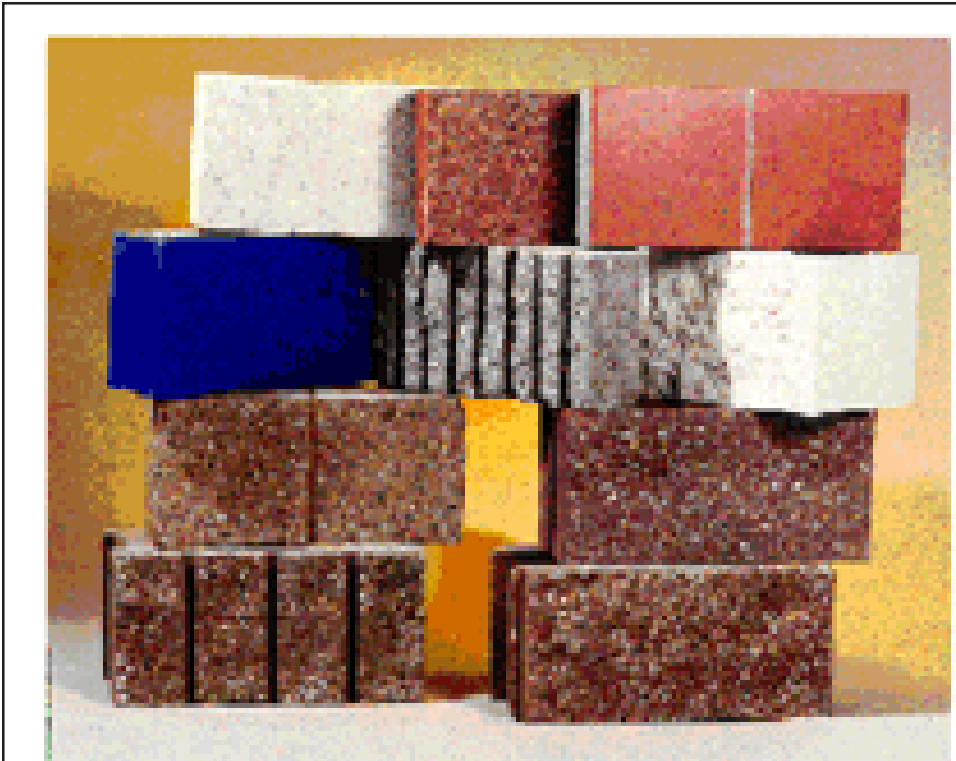
Figure 7—Examples of Surface Finishes Available For Concrete Masonry Units (clockwise from bottom left: split face with three scores; single score ground face; glazed corner unit; ground face; ground face; single score glazed ; split face; ground face; split face; center: eight-ribbed split face)
